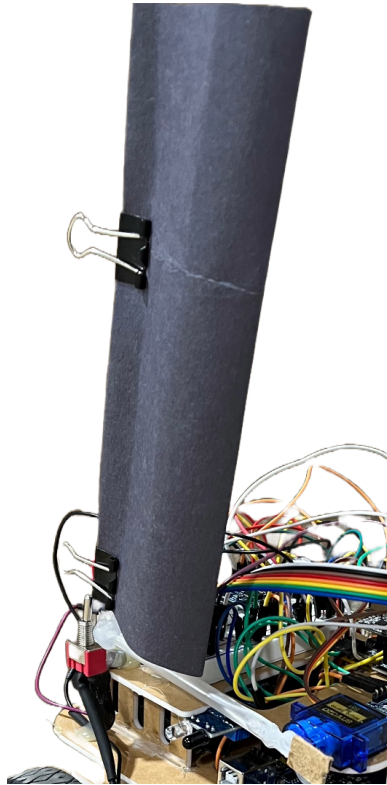
Figure 3: Photo of the TRIDENT ladder assembly, featuring a flexible, black paper arm clipped onto a plastic straw.
